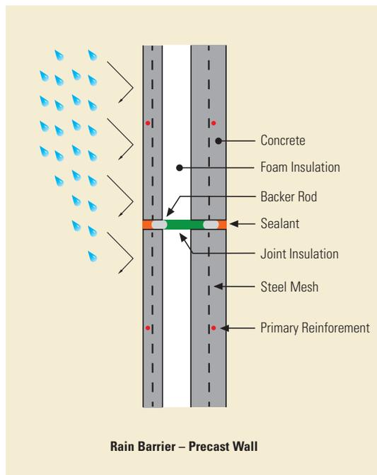
*The high tensile strength of reinforced concrete combined with proper compaction imbues the material with the capacity to withstand storms and render it resistant to wind-driven rain and moist outdoor air in hot and humid climates.*
