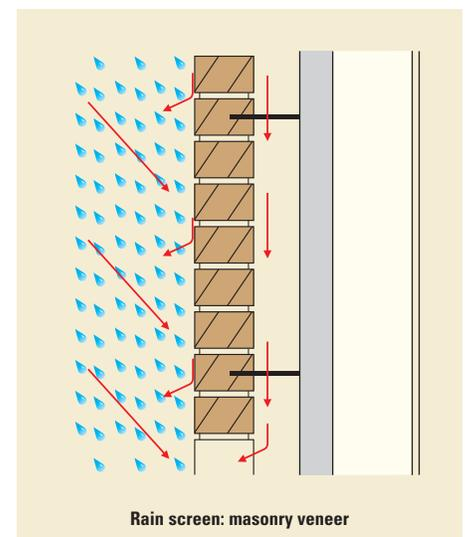
**Above:** Rain screens permit moisture to penetrate the exterior wall system. They must be designed to drain the water back to the exterior, which often requires complicated engineering and construction practices.
