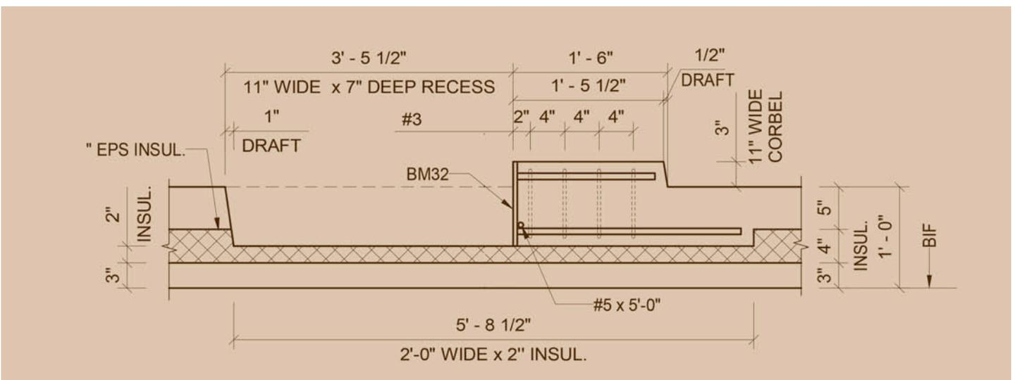
**Figure 8** Bearing enlargement section
