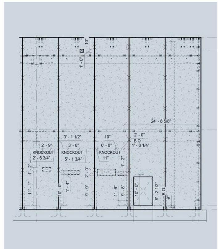
Figure 3 Partial elevation of non-loadbearing wall (56–10½" tall)
