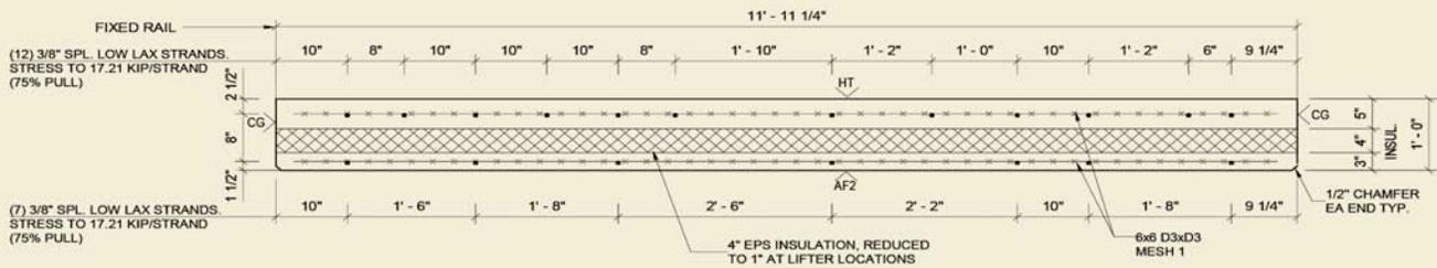
Figure 5 Wall section
