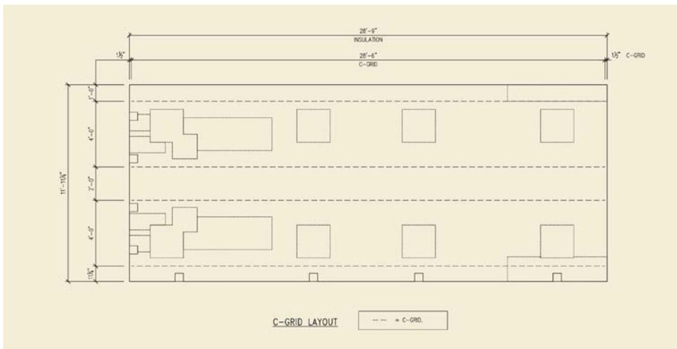
Figure 10 C-GRID layout for loadbearing wall
