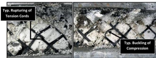
Fig. 6: Typical Observed Failure of the CFRP Grids
