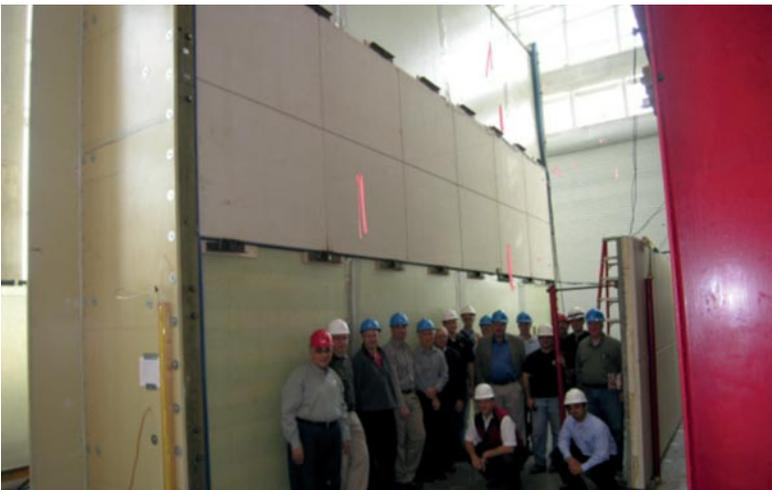
*Fig. 15: Precast Composite Sandwich Panel in Uniform Pressure Chamber after Sustaining (Factored Load in Both Directions without Cracking)*
