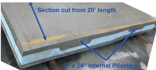
Fig. 7: Cross-section of 6.1 m (20-ft) tall Panels Showing Two Internal Pilasters
